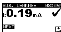
Figure 6.32: Substitute leakage result screen
