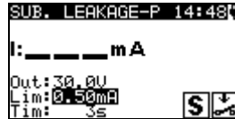
Figure 6.37: Substitute leakage - P starting screen
