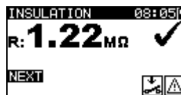
Figure 6.30: Insulation result screen
