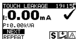
Figure 6.18: VDE Organizer – Touch leakage result screen
