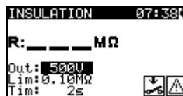
Figure 6.29: Insulation resistance starting screen
