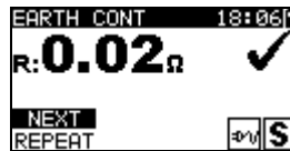
Figure 6.28: Earth continuity result screen
