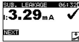
Figure 6.9: VDE Organizer – Substitute leakage result screen
