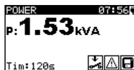
Figure 5.40: Example of apparent power measurement result
