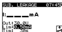
Figure 6.31: Substitute leakage starting screen
