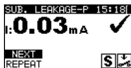
Figure 6.16: VDE Organizer – Substitute leakage - P result screen
