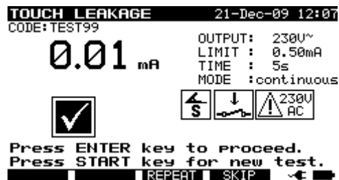
Touch leakage test menu
