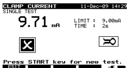
Examples of clamp current measurement result
