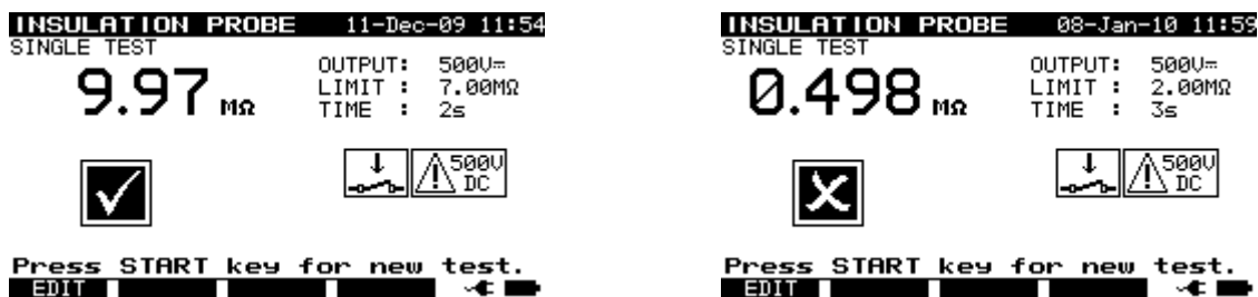
Example of insulation-S probe resistance measurement results
