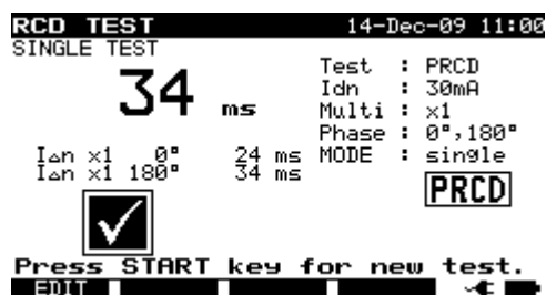
Examples of RCD test result
