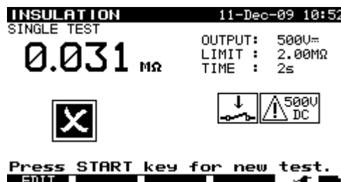
Examples of insulation resistance measurement results
