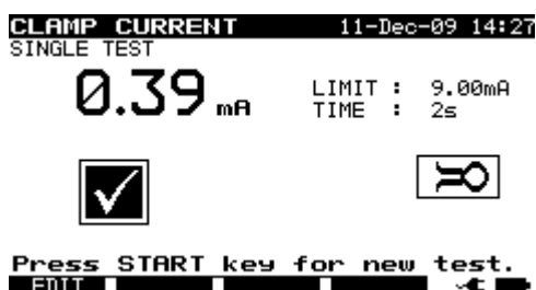
Examples of clamp current measurement result
