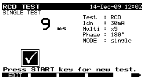
Examples of RCD test result
