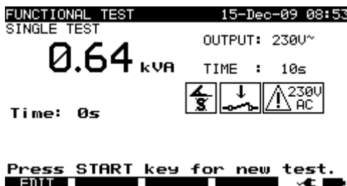
Example of apparent power measurement result
