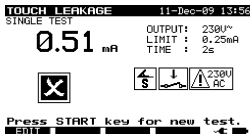
Examples of touch leakage current measurement results
