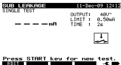
Sub leakage menu
