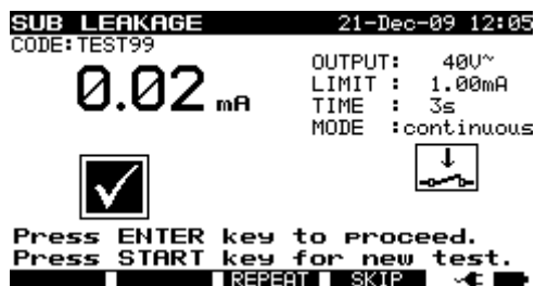
Substitute leakage test menu
