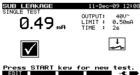
Example of substitute leakage current measurement results
