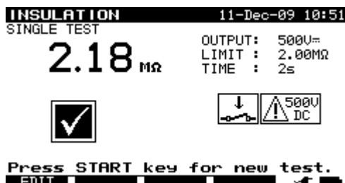
Examples of insulation resistance measurement results
