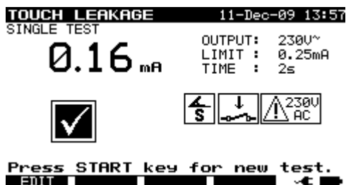
Examples of touch leakage current measurement results
