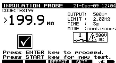
Insulation resistance – S probe menu
