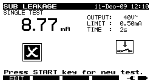
Example of substitute leakage current measurement results
