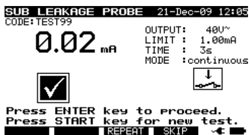
Substitute leakage - S test menu
